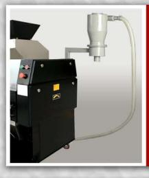
MACHTEK Plastic Granulator MG15A comes with a blower and cyclone dust separator or with a practical bin.
