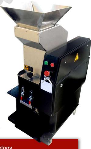
Plastic Granulator MG 15A is designed with CSCG technology which guarantees continuous operation, perfect sealing of cutterhouse for low noise and dust and uniform regrind size with a minimum of dust and fines.
