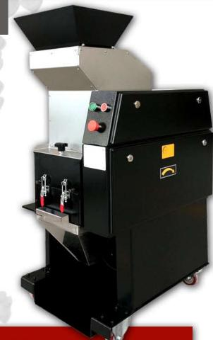
Plastic Granulator MG 15B is designed with CSCG technology which guarantees continuous operation, perfect sealing of cutterhouse for low noise and dust and uniform regrind size with a minimum of dust and fines.
